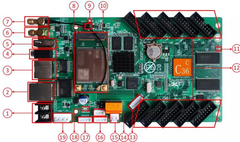
1. Power Supply port: connected 5V DC power supply.
