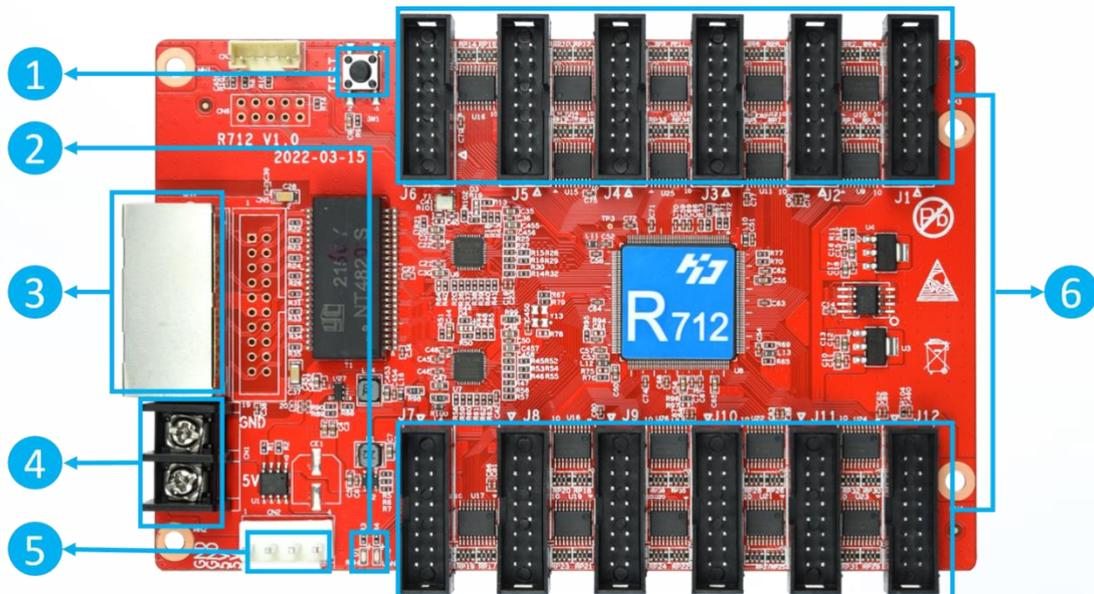
①: Test button, used to test display brightness uniformity and display module flatness.
