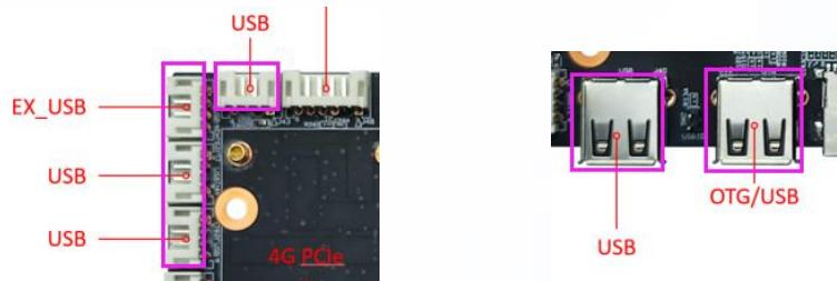
The board has 2 USB standard interfaces (the left one is device mode), 2 built-in USB sockets for peripheral expansion.
