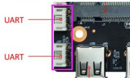
The board have to two sets of ordinary UART serial ports, which can support the UART serial port devices on the market.
