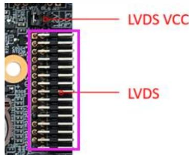
General LVDS interface definition, support single / dual, 6/8 / 10-bit 1080P LVDS screen. The screen voltage can be selected through a jumper cap, and it can be selected to support 3.3V / 5V / 12V screen power supply.
