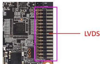
General LVDS interface definition, support single / dual, 6/8 / 10-bit 1080P LVDS screen. The screen voltage can be selected through a jumper cap, and it can be selected to support 3.3V / 5V / 12V screen power supply.
