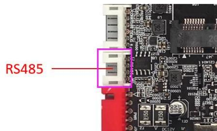
1 group of 485 communication interface, which can support common 485 interface equipment on the market. The level of the interface is 5V. If the level of the connected interface is higher than 5V, there must be an isolation circuit or a level conversion circuit, otherwise the main control and equipment will be burned out.
