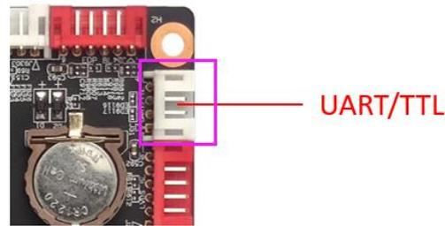
1 set of ordinary two-wire serial ports, which can support common serial devices on the market. The level of the serial ports is 0V to 3.3V. If the level of the connected serial port is higher than 3.3V, there must be an isolation circuit or a level conversion circuit, otherwise the main control and equipment will be burned out.
