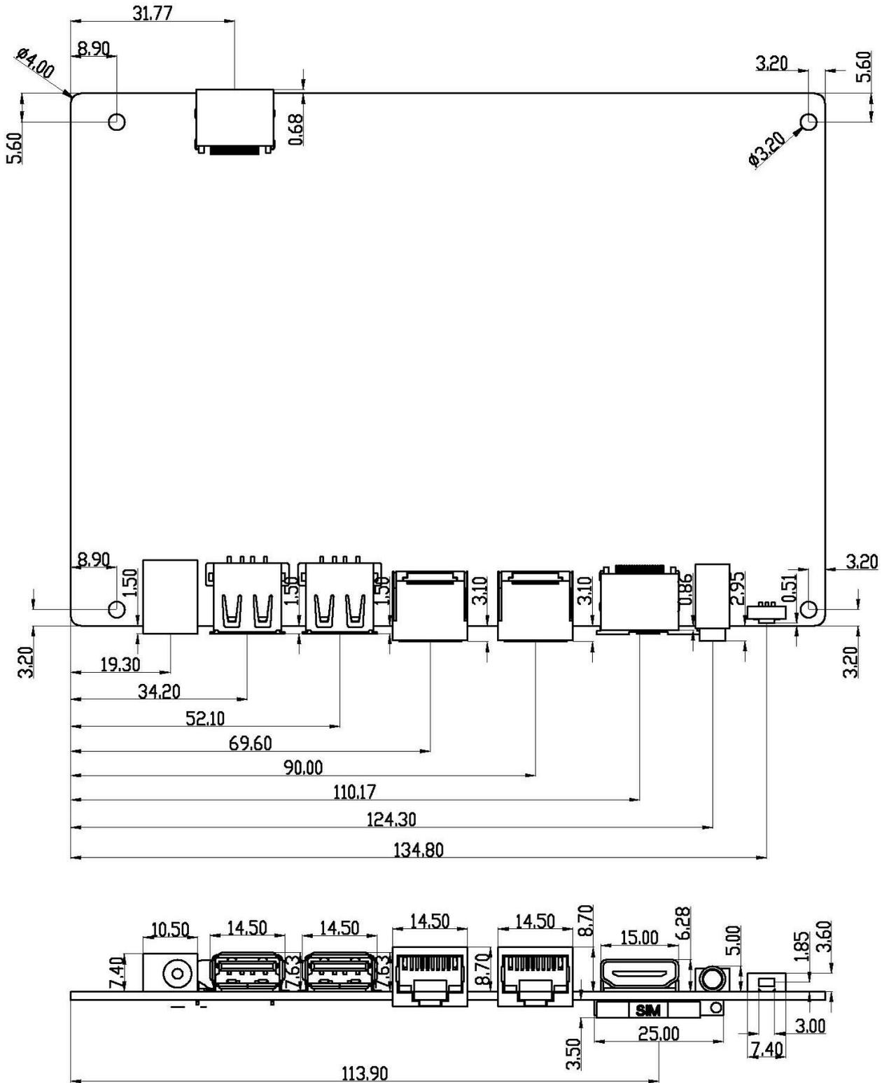
Screw hole specifications:  $\phi 3.5\text{mm} \times 4$
