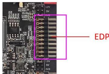
This interface is a common EDP screen interface, in the form of 10 \* 2 double row pins, can optional 3.3V/5V/12V screen power supply.
