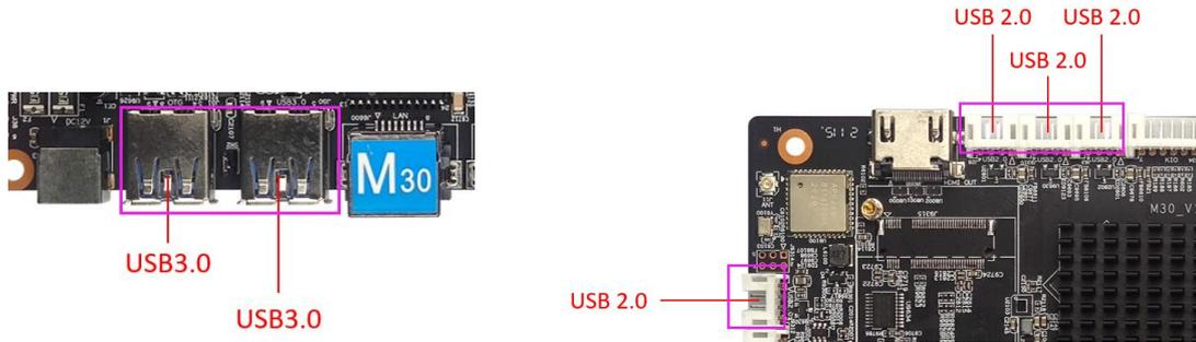
The board has 2 USB 3.0 standard interfaces, 4 build-in USB2.0 sockets for peripheral expansion.
